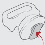
All tie-downs equipped with t-bolts for track mounting
